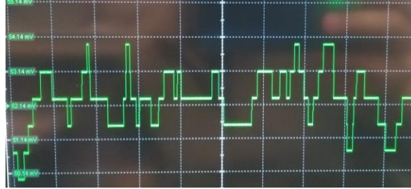
Fig. 2.6: Received PAM signal after fiber transmission.
