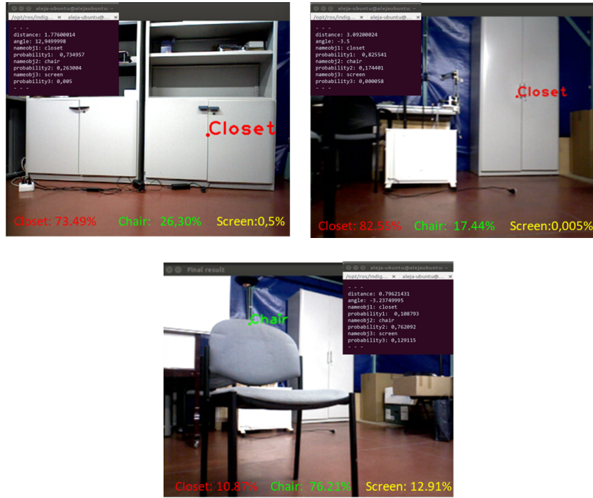
Figure 3.4: Results of the object detection model applying uncertainties. The experiment has been carried out in a laboratory at the University Carlos III of Madrid. The label of the detected object is displayed in each image frame.
