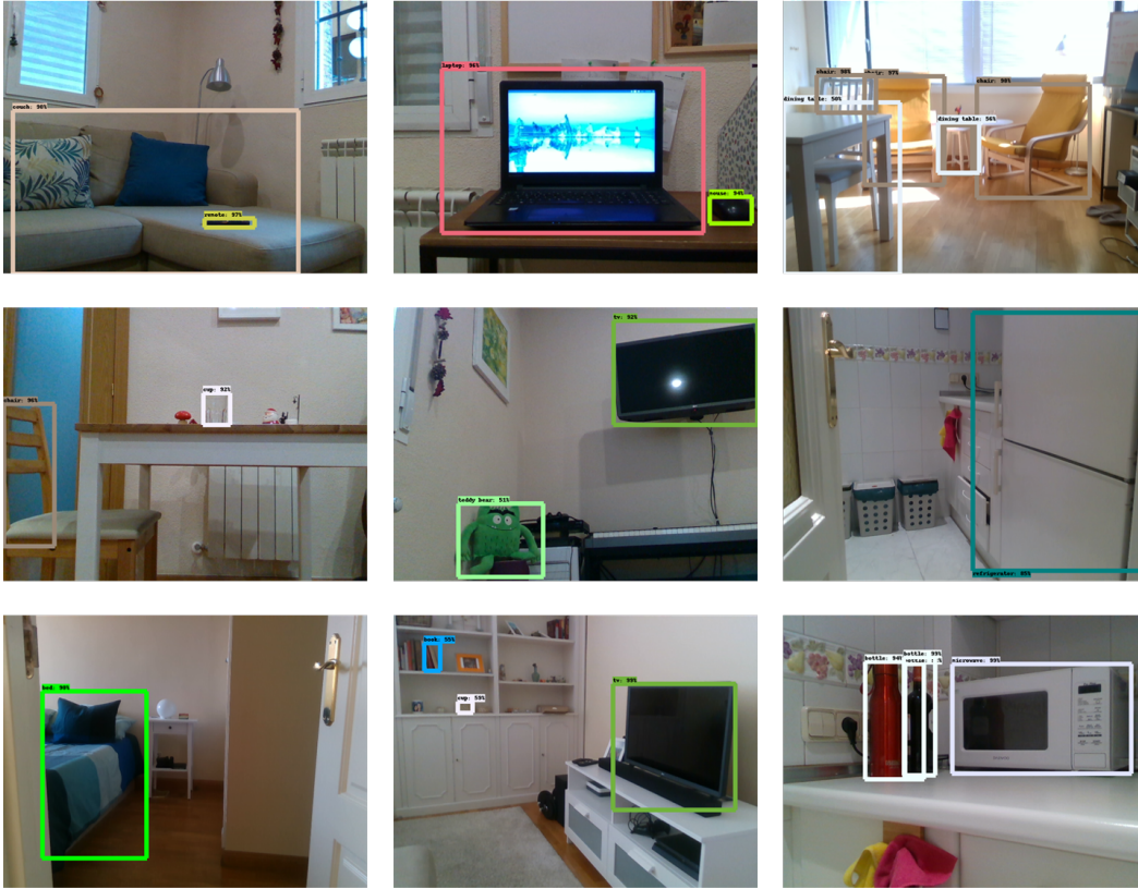
Figure 3.6: Results of object detection model based on deep learning techniques. Each detected object is enclosed in a bounding box with the detection confidence of the underlying object category.
