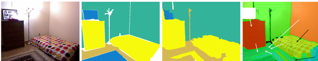
Figure 2.1: Instant segmentation and semantic labeling of single images presented in [205]. The method based on MRF segments images into regions and infer support relationships.
