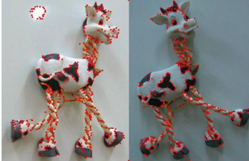
Figure 2.2: Keypoints detected for the same object under an image transformation using the Harris corner detector [9].
