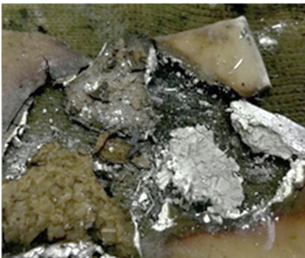
Fig. 12 – Macrograph of carbonized wastes of UPE after fire test of any sample (Picture after a fire test for 30 min of +50M + 3GF bio-composite).
