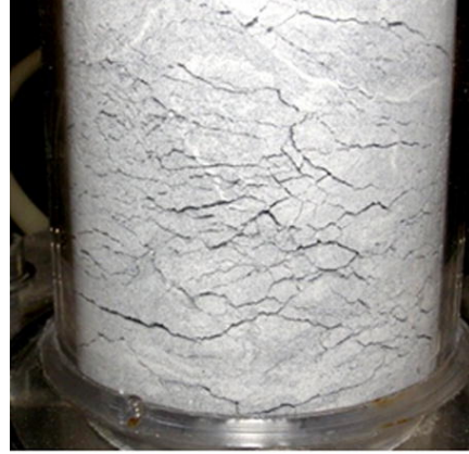
(b) Fissures in the bed
