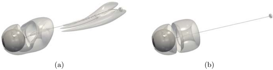
FIGURE 15: Instantaneous visualization of the flow structures around the sphere with the deformable filament at (a) initial time instants, and (b) after reaching and stable state. Vortical structures correspond to iso-contours of the Q -criterion, Q = 0.2U^2/D^2 , as in Fig. 13.
