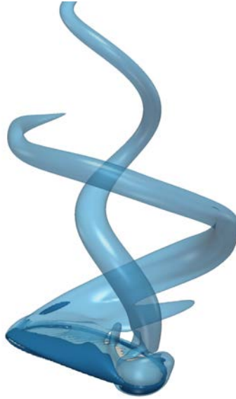
FIGURE 5: Iso-surfaces of the Q -criterion for Re = 240 . Light blue iso-surface \tilde{Q} = 0.5 , dark blue iso-surface \tilde{Q} = 5 , where \tilde{Q} = Qc^2/w_d^2 .
