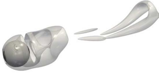
FIGURE 13: Instantaneous visualization of the flow structures around the isolated sphere at Re = 300 . Vortical structures correspond to iso-contours of the Q -criterion, Q = 0.2U^2/D^2 .
