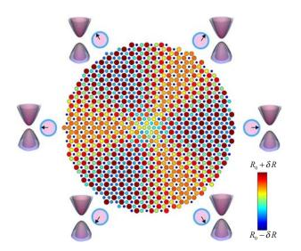
FIG. 1. An acoustic analog of a topological superconductor vortex made of rigid cylinders of varying radii, arranged in a finite triangular sonic lattice. The color of the cylinders illustrates the radius distortion  $R_0 \pm \delta R$ , as given by Eq. (2). The Kekulé phase  $\phi$ , together with the local intervalley gap as one moving around the vortex, are depicted around the perimeter.
