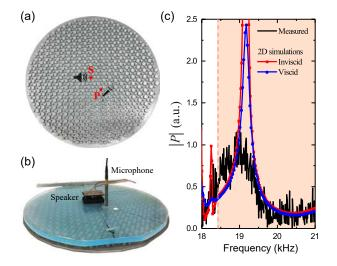
FIG. 4. (a) Photograph of the 3D printed Kekulé distorted sonic lattice, with parameters n = 1, d = 9 mm,  $R_0 = 0.35d$ ,  $\delta R = 0.15d$ ,  $\xi = 2a$ , and  $a = \sqrt{3}d$ . (b) A rigid lid was mounted above the cluster into which holes were drilled to fasten the speaker and the microphone. (c) The spectrally measured pressure at point *P* (black) is compared to both inviscid (red) and viscid (blue) numerical computations in near proximity to the edge of the band gap.
