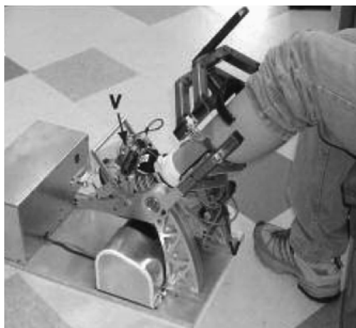
FIGURE 1.15: Assisted Movement With Enhanced Sensation (AMES) [Cordo et al., 2009]. (Permission is granted at no cost for use of content in a Master's Thesis and/or Doctoral Dissertation.)
