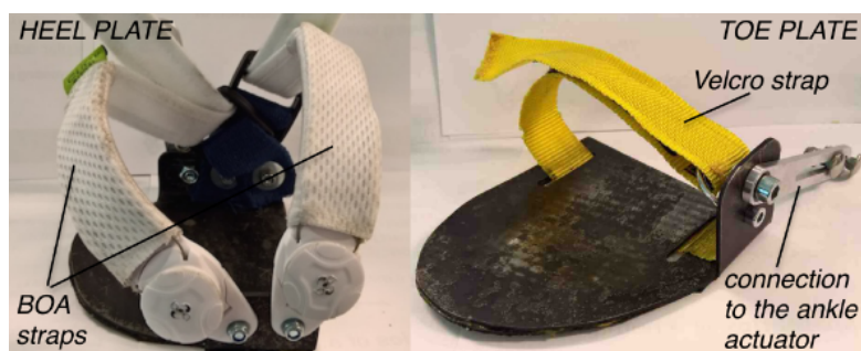
FIGURE 2.7: The plates have a low footprint and are easily adjustable to different users. Two BOA straps are used at the heel plate, and a single Velcro strap at the toe plate. Both plates are slightly bent up on one side - toe plate at the toe side, heel plate at the heel side, to allow a more natural walking pattern. Intermediary links and carriage screws are used to fix the plates to a desired position with respect to the ankle actuator (and thus ankle joint axis). Copyright ©2017, IEEE
