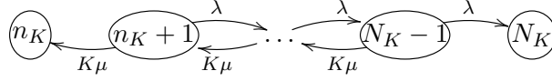
Figure 4.4: CTMC for Stage K : K active APs and no AP powering on
