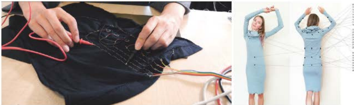
Fig 2. Left: first prototype of Magic Lining , allowing the user to experience a series of vibration motors delivering sensation patterns to the body through textile. Right: The vibration motor positioning on the final prototype. For a video describing the project and process: https://vimeo.com/289294125
