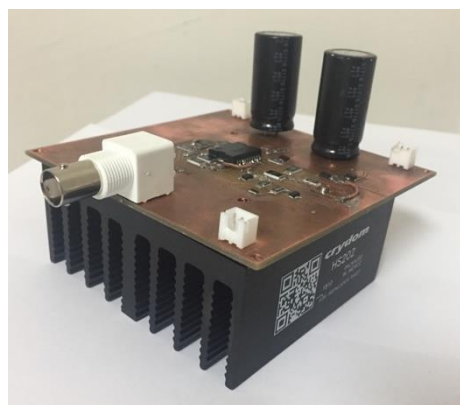
Figure 43. Heat sink HS202 screwed to the PCB
