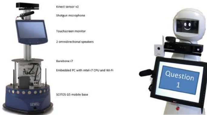
Fig. 1. The robot used for CGA, showing sensors (left) and shell (right).
