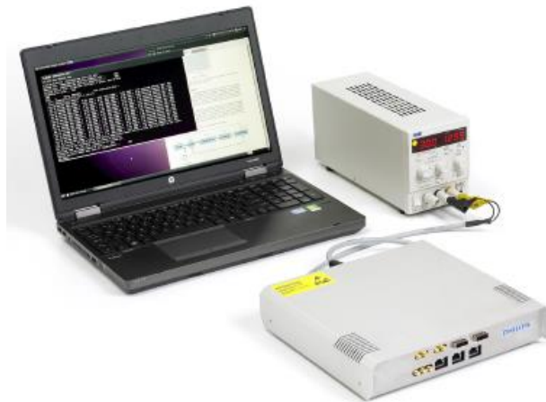
Figure 50: Image showing the laptop, power supply and base unit of the PDPC-module-TEK [35]
