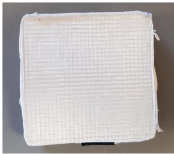
Figure 66: 30x30 LYSO scintillator
