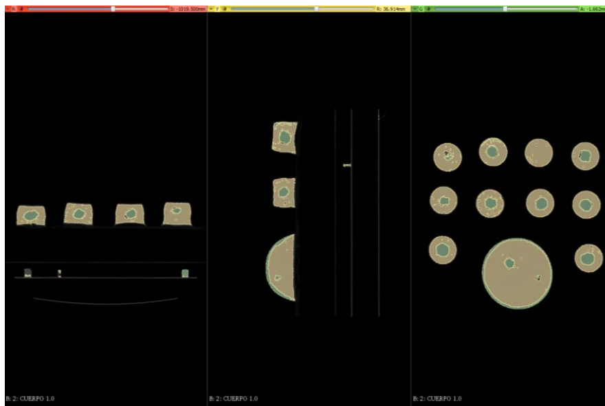
Fig. 35. Intensity thresholding segmentation in 3D Slicer of the tumor and the breast mimicking tissue from the CT images of the manufactured phantoms.
