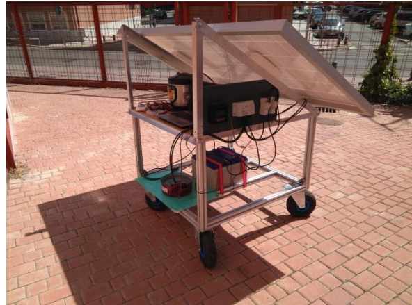
Figure 16. Photovoltaic system seen from the side.
