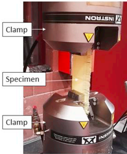
Fig. 5. (a) Set-up for the fabric tensile test. (b) Example of the five tests carried out for fabric F.
