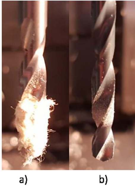
Fig. 9. Drills after performing a hole at a cutting speed of 23 m/min and a feed of 0.025 mm/rev; a) Brad & Spur and b) Twist respectively.
