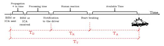
Fig. 3: Time-line describing the communication between vehicles.
