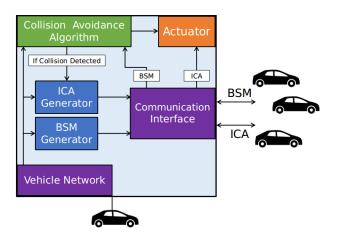
Fig. 1: Vehicle's OBU logic blocks.
