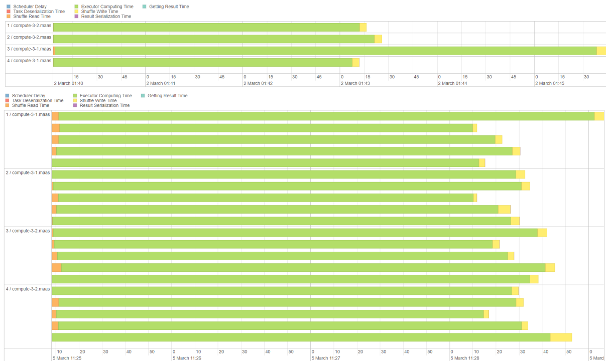
Figure 7.19: Timeline for the projection component on a distributed GPU-based cluster for Configuration A, 4 executors with one core (top) and Configuration B, 4 executors with 5 cores (down).
