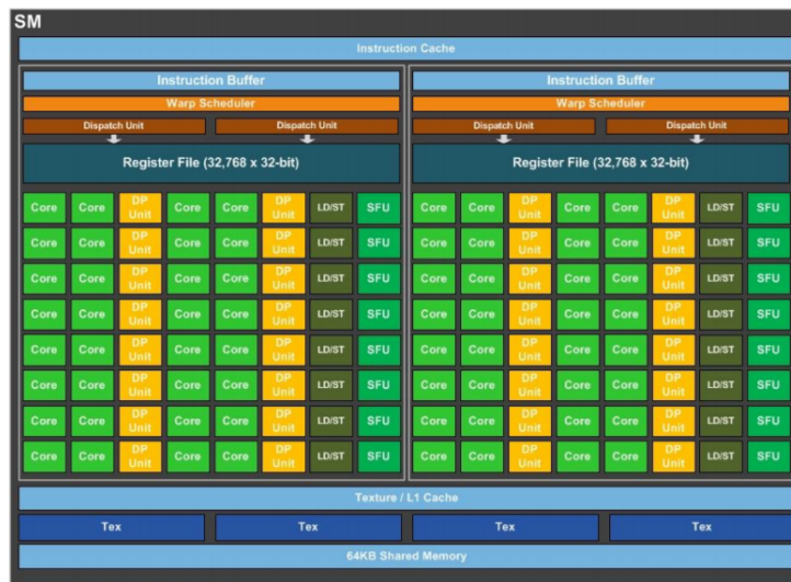
Figure 2.4: Pascal architecture for the SM, NVidia [28].
