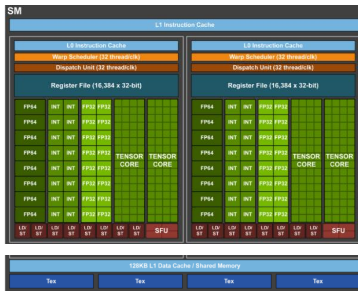
Figure 2.5: Volta architecture for the SM, NVidia [29].
