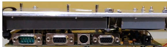
Figure 3. Profile view of the shielding between the PCB and the cover of the filter box.
