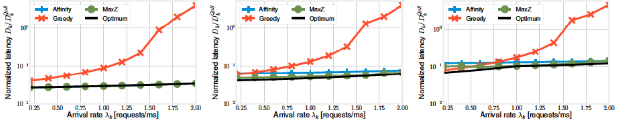
Fig. 5. Normalized latency (log scale) as a function of arrival rate \lambda for the chain (left), light mesh (center), heavy mesh (right) VNF graphs.
