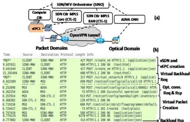
Fig. 7. (a) Setup between CTTC SDN/NFV orchestrator and the ADVA ONH.; (b) Capture of the control messages for setting up the VNFs and backhaul.
