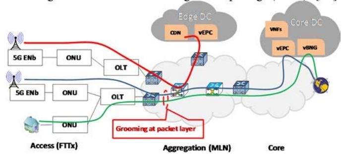
Fig. 2. Multiple fixed and mobile services in a converged MLN
