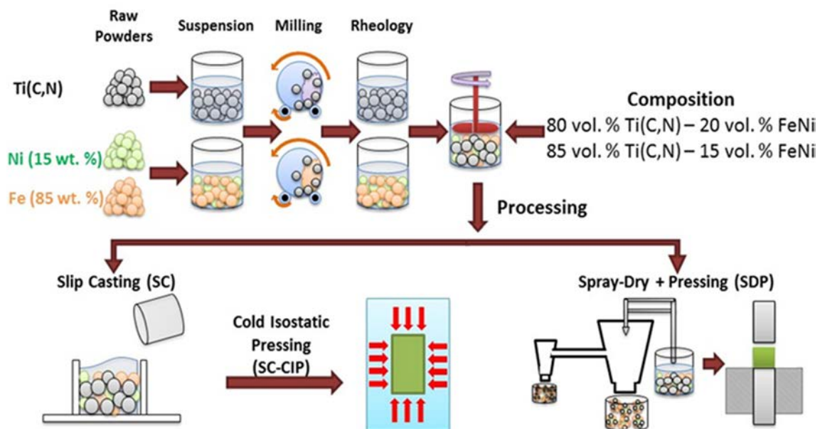
Fig. 1. Schematic of the different processing routes including the steps of slurry preparation as well as the employed processes of shaping/compacting.
