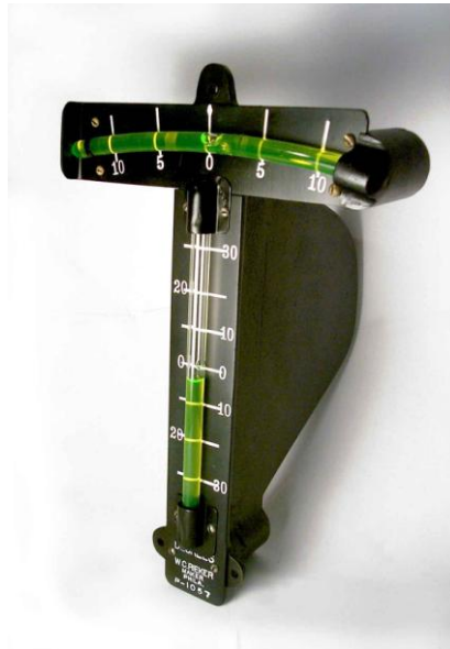
Illustration 3. Spirit of Saint Louis bubble inclinometer
