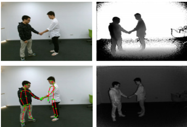
Fig. 5 Some samples of RGB, depth, skeleton and IR image from the NTU RGB+D dataset [179].
