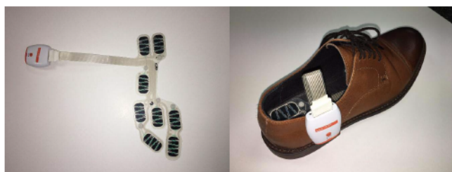
Fig. 1. Smart Insole Technology: Left - FSRs showing a typical layout, Right - Donning arrangements of ankle strap and accompanying footwear.
