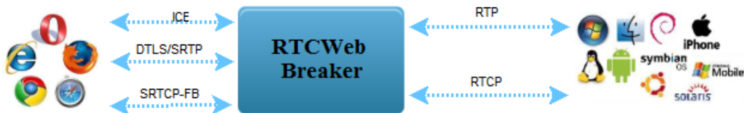
Figure 2.10: WebRTC2SIP RTCWeb Breaker architecture [8]
