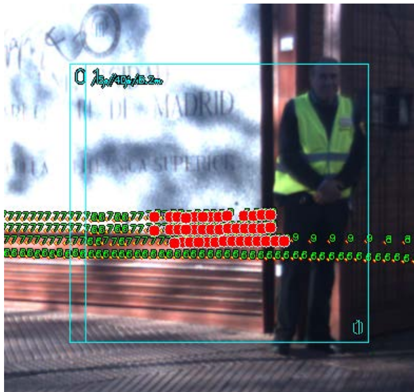
Fig. 91 ROI overlapping due to close detections (clusters are displaced to the left for better displaying).
