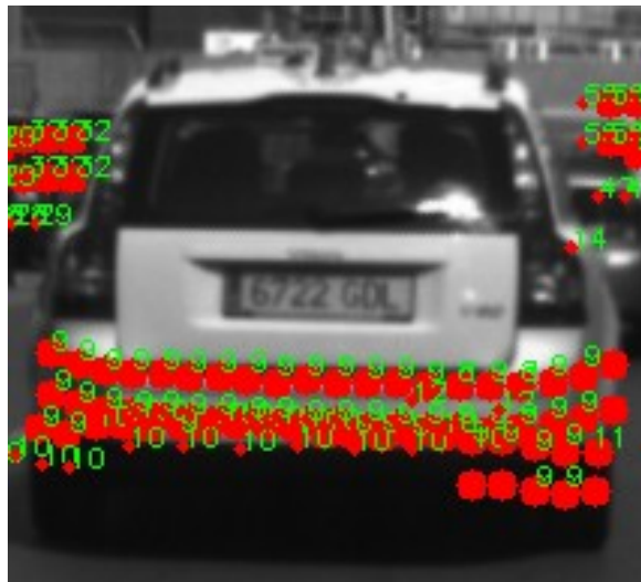
Fig. 33 Obstacle detection, represented as a cluster.
