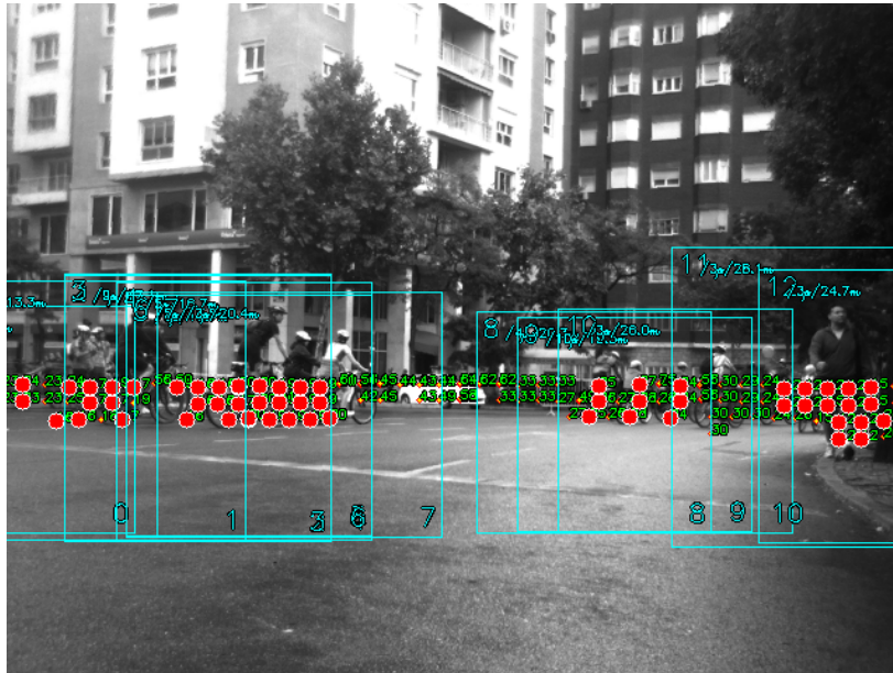
Fig. 11 Cluster extraction and ROI generation in image. Red dots represent the clusters found, and blue squares are the ROIs for bicycles search using computer vision algorithms.
