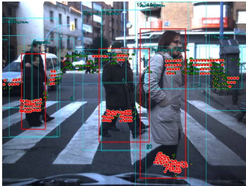
Fig. 92 Example of pedestrian classification. Blue squares are obstacle detections, big red dots are clusters, red squares are sensor fusion pedestrian positive classifications.
