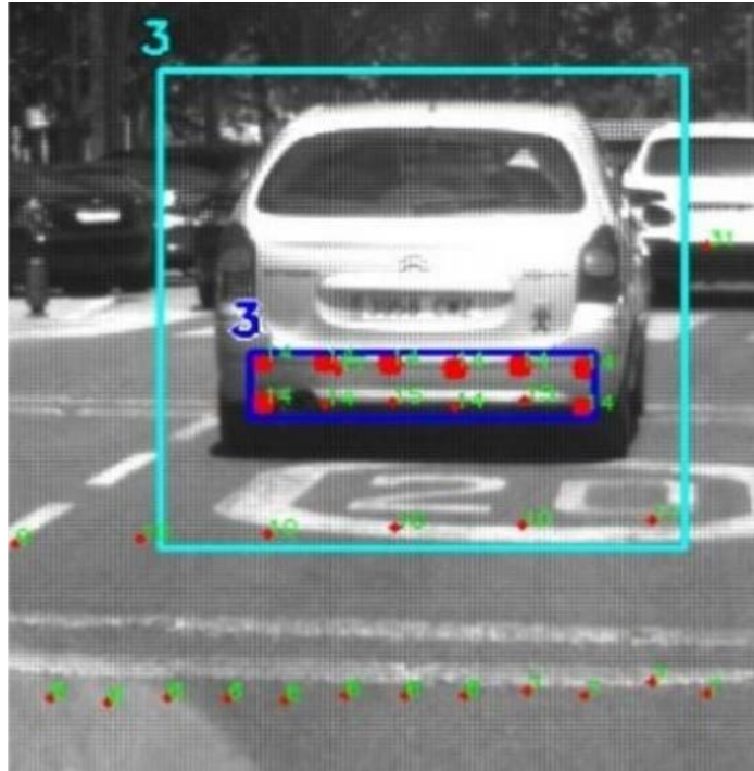
Fig. 37 Cluster removal in ground plane. Points in the bottom of the image meet the geometrical constraints for cluster creation, but are omitted because of ground plane belonging.
