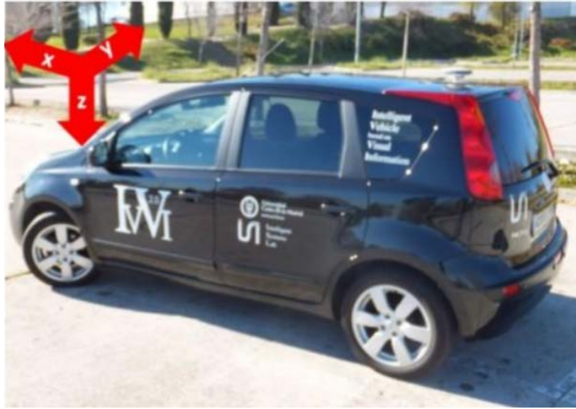
Fig. 35 IVVI 2.0 research platform with axis represented in the image: X=laser-obstacle distance, Z=detection height, Y=horizontal deviation from the laser.
