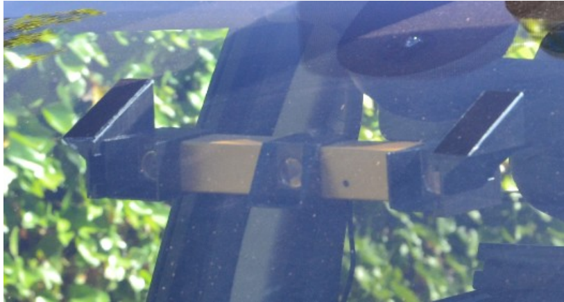
Fig. 30 Bumblebee XB3 camera installation in the IVVI 2.0.
