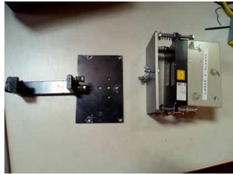
(b) Metal bracket and orientation system
