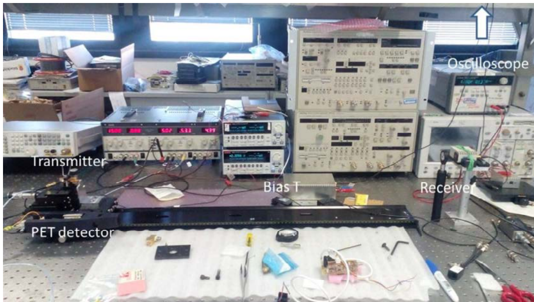
Figure 7.4 Experimental setting of transmission of PET analog pulses over OWC.
