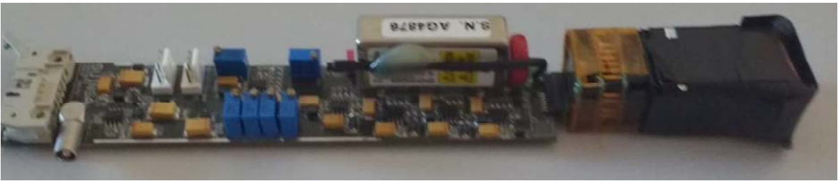
Figure 4.1 Argus detector element with a scintillator mounted on the PMT (right)
