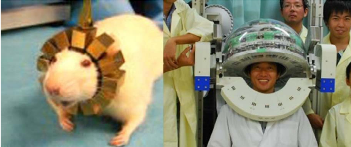
Figure 2. 14 (Left) RatCAP, conscious rodent brain PET scanner; and (right) human brain PET [51].
