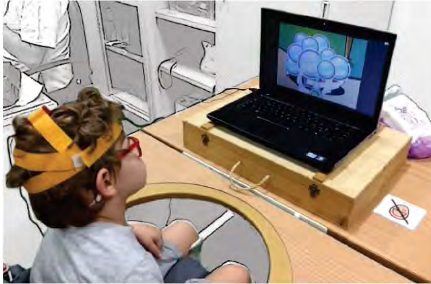
FIGURE 3.3: A training session with ENLAZA. The user has a wired IMU attached to a headset and plays the game Look2Learn (Sensory Software International Ltd.).
