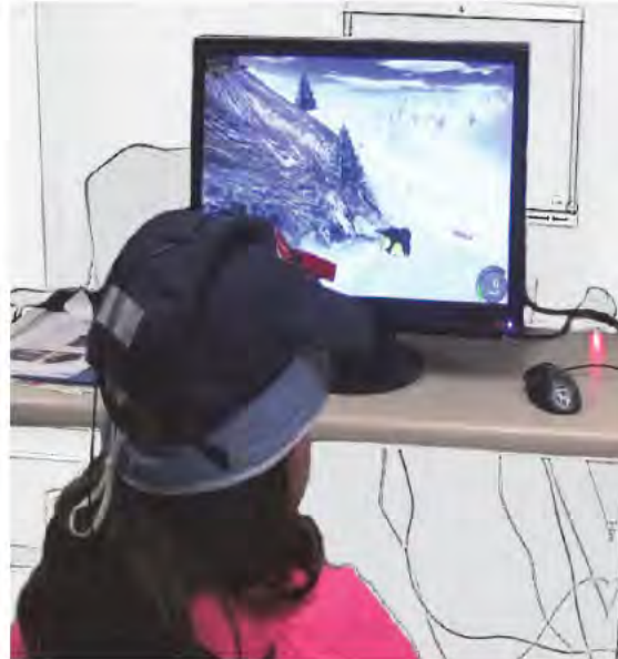
FIGURE 5.3: A training session with ENLAZA. The user has a wired IMU attached to a baseball cap and plays the game Extreme Tux Racer.
