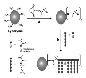
Scheme 3 Synthetic strategy for the lysozyme-*N*-hydroxysuccinimide initiator and subsequent living radical polymerisation of PEGMA<sub>475</sub> and rhodamine monomer. Reagents and conditions: (a) Phosphate buffer (100 mM, pH = 7.0), DMSO/TEA (95/5; v/v), 25 °C, 48 h; (b) Cu(I)Br/*N*-(Ethyl)-2-pyridylmethanimine, PEGMA<sub>475</sub>, Rhodamine B methacrylate, H<sub>2</sub>O, 25 °C, N<sub>2</sub>, 48 h.
