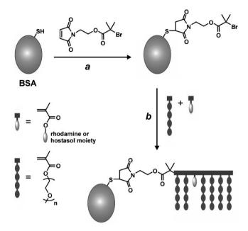
Scheme 2 Synthetic strategy for the BSA–maleimide macroinitiator and subsequent living radical polymerisation of PEGMA<sub>475</sub> and fluorescent monomers. Reagents and conditions: (a) phosphate buffer (100 mM, pH = 7.0)/DMSO (96/4; v/v), 25 °C, 12 h; (b) Cu(1)Br/*N*-(ethyl)-2-pyridylmethanimine, PEGMA<sub>475</sub>, Rhodamine B methacrylate, H<sub>2</sub>O, 25 °C, N<sub>2</sub>, 48 h.
