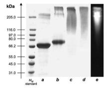
**Fig. 1** SDS-PAGE of native BSA (a), BSA-macroinitiator (b), BSA-poly(DMAEMA-*co*-rhodamine) (c), BSA-poly(PEGMA<sub>475</sub>-*co*-rhodamine) (d) and BSA-poly(PEGMA<sub>475</sub>-*co*-rhodamine) under UV at  $\lambda$  = 302 nm (e).
