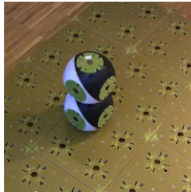
Figure 2.27: A single RB module in a 2D grid world, where each grid contains an ACM connector. Source: [Bonardi et al., 2012]
