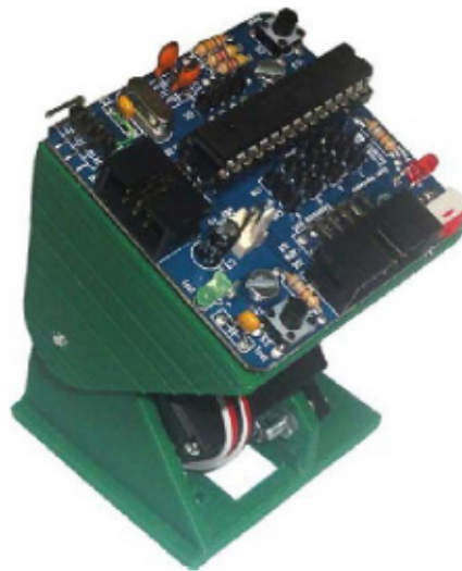
Figure 5.4: SkyMega board mounted on a Y1 module. Source:
