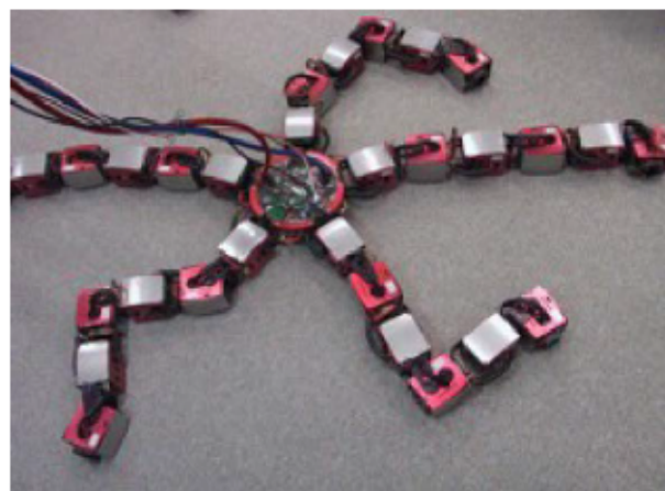
Figure 2.25: The Brittle Star MR, with five limbs and six modules per limb. Source: [Lal et al., 2006]
