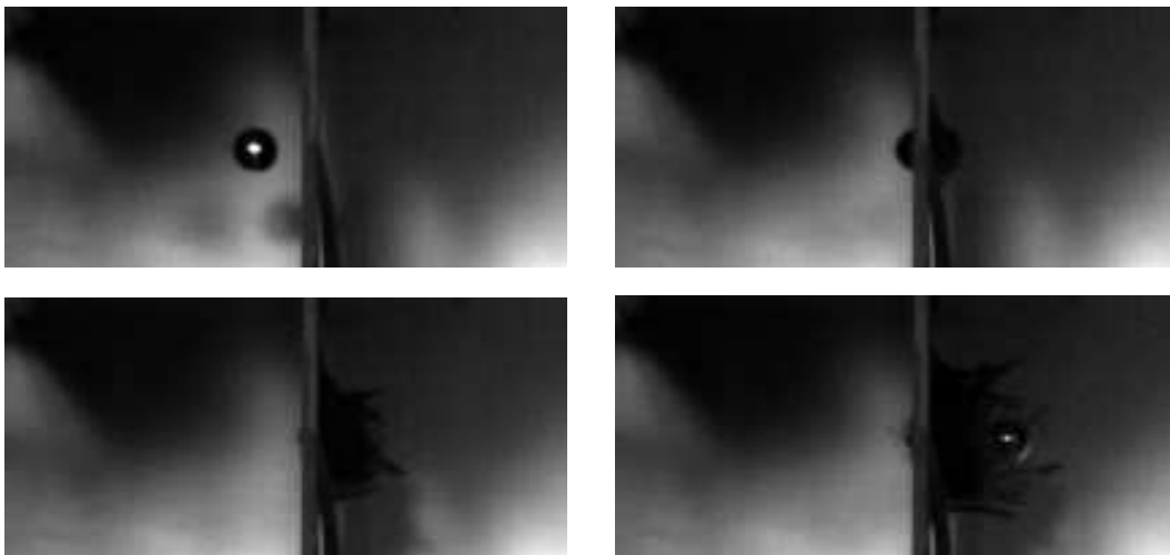
Fig. 1. Impact sequence from a normal impact at 223 m/s.
