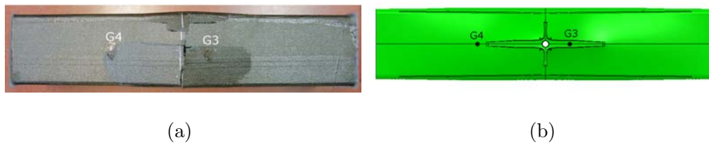
Fig. 13. Final failure at the exit wall of the CFRP tube. v = 900 \text{ m/s}
