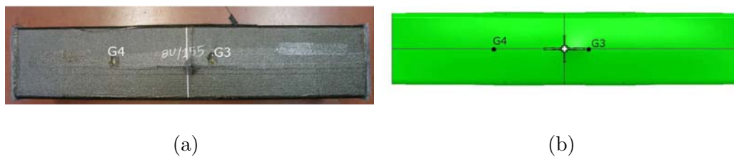
Fig. 14. Final failure at the exit wall of the CFRP tube. v = 600 \text{ m/s}
