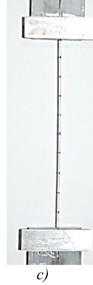
Figure 1: (a) POF fibre geometry, (b) specimen mounting scheme, (c) specimen showing the dot markings
