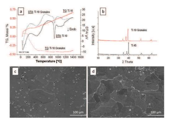
**Figure 3.** (a) DTA-TG curves of Ti10 initial powder and agglomerates obtained by spray-dry. (b) XRD patterns of sintered samples obtained from Ti45 as-received powder and Ti10 granules. (c) Microstructure of sintered samples obtained from Ti45 as-received powder. (d) Microstructure of sintered samples obtained from Ti10 spray-dried powders, pressed and sintered in the same conditions than (c) (1100 °C, 30 min, vacuum).
