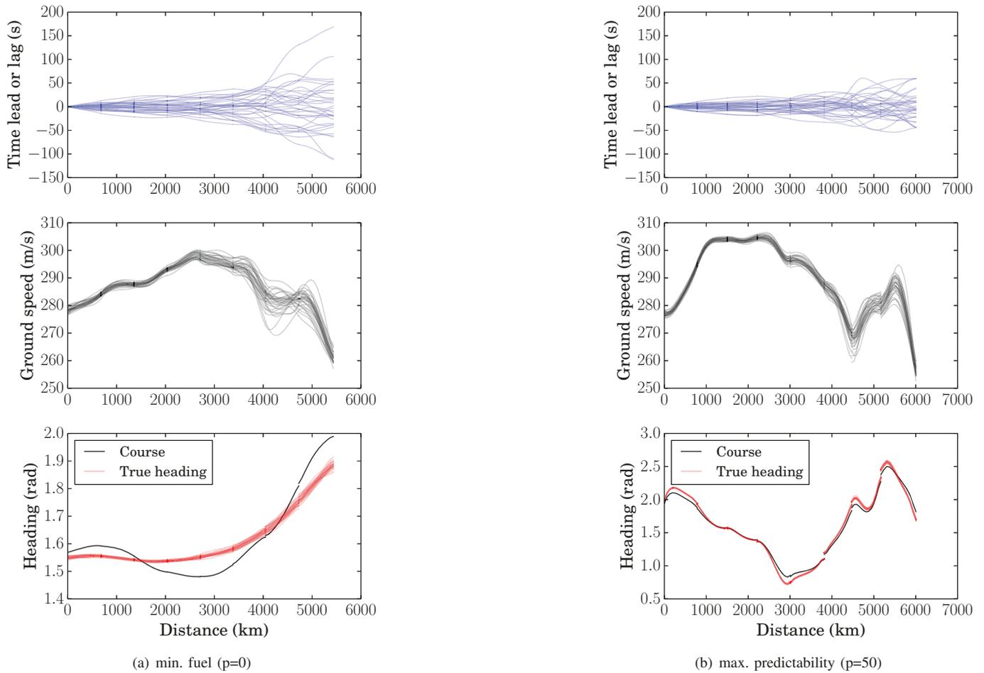
Figure 4. State-space evolution of the variables in the case  $p = 0$  and  $p = 50$ . Time leads and lags are defined with respect to the average trajectory.
