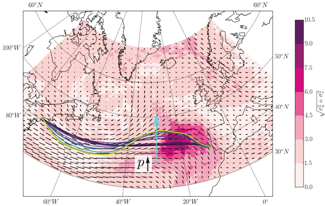
Figure 3. Optimal trajectories from NY to Lisbon, for values of  $p$  from 0 to 50. Higher brightness in the trajectory color indicates higher values of  $p$ . We also color regions of higher uncertainty, which we have defined as  $\sqrt{\sigma_u^2 + \sigma_v^2}$ , with  $\sigma_u$  being the standard deviation of the  $u$  component of wind across different members and  $\sigma_v$  analogous for the  $v$ -component.
