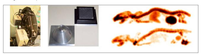
LEFT: Photograph of the r-SPECT prototype. Center: parallel and pinhole collimators. Right top: MIPS render of a 24 g mouse bone scan (99mTc-MDP) using pinhole collimators. Right bottom: MIPS render of a 150 g rat scanned using the same compound and parallel-hole collimators
