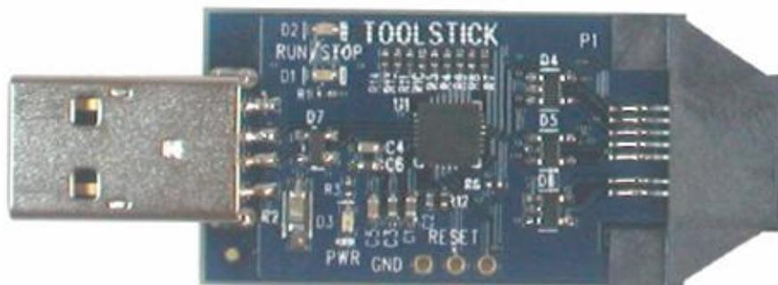
**Figura 3.15.** *Toolstick Base Adapter.*
