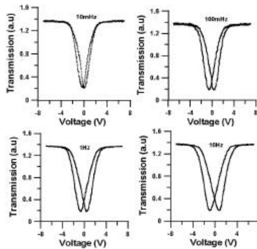
Fig. 2. Optical transmission for different frequencies of the triangular waveform applied to the LC cell.
