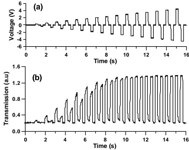
Fig. 4. (a) Driving waveform and (b) the gray scale obtained in the time domain.
