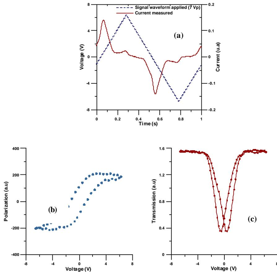
Fig. 7. (a) Triangular waveform applied to the cell and measured switching current, (b) polarization-voltage characteristic obtained, and (c) W-shaped optical transmission measured for the LC device studied.
