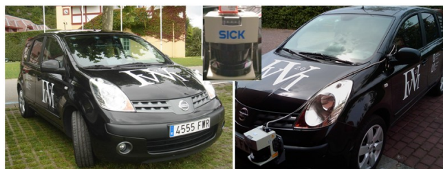
Figure 1. Test platform IVVI 2.0. (Intelligent Vehicle based on Visual Information). Left the vehicle. Right the laser scanner mounted in the bumper of the vehicle. Center, closer look of the laser scanner sensor.
