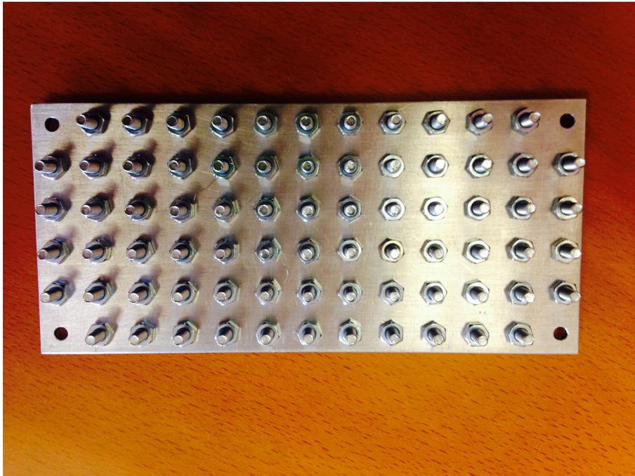
Figura 6.7: **Bed of nails** low cost
