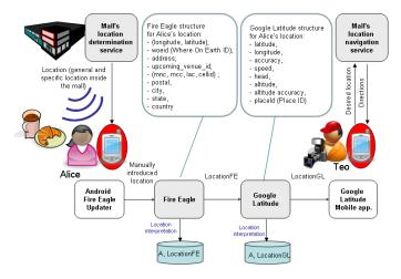
Fig. 5. Illustration of the interoperable hierarchical structure for location information use case: Current representation of location information in each location-based web service.
