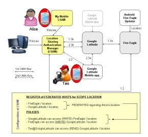
Fig. 3. Illustration of the user-managed sharing between multiple hosts use case: Entities and their interactions for the PUSH mode
