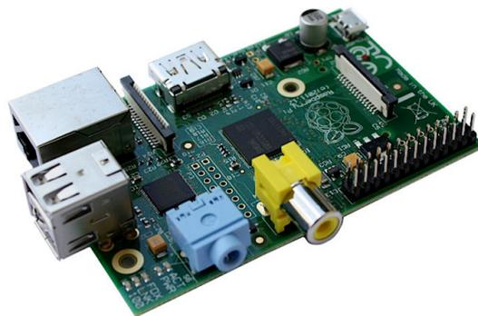
Figura 3.4: Raspberry Pi modelo B.[22]
