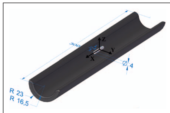
Figure 3. Geometrical definition and coordinate system. Magnet polarization direction parallel to X direction.
