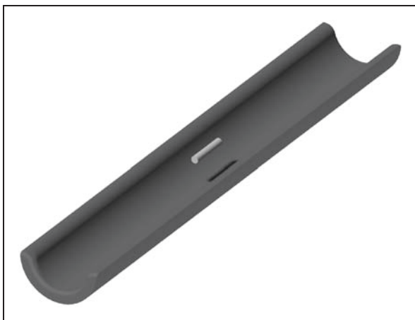
Figure 1. Drawing of the linear bearing: Magnet over a superconductor in the Meissner state.
