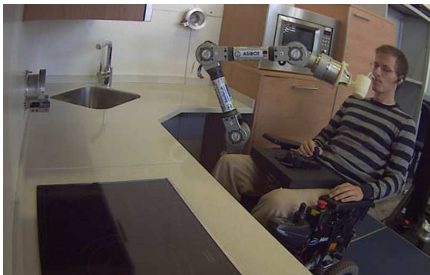
Fig. 1. The ASIBOT robot attached to the wheelchair DS in the kitchen test-bed at UC3M. Two fixed DS can be seen mounted on the walls.
