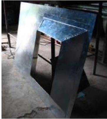
The back cover of the oven has to be adapted for the receiver window.
